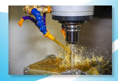
Nearly all machining operations create oil mist, the aerosol formed when oil is used for cooling or lubricating during the machining of metal or plastic components. Proper ventilation is required to prevent oil mists from fouling equipment, products, and the working environment.
